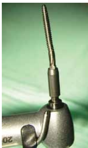
FIG. 2 Severe implant deformation after removal.
